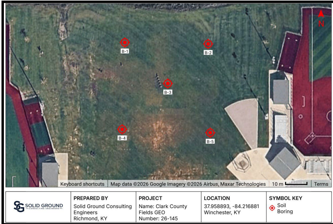
Figure 15: Approximate Boring Locations: High School
